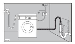
The drain hose may be extended to a maximum of 4 metres. An additional drain hose and joining piece is available from your local Service Force Centre.
